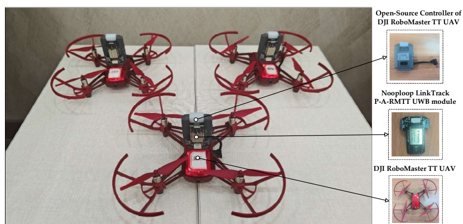
Figure 6. Experimental UAV and its associated equipment.
