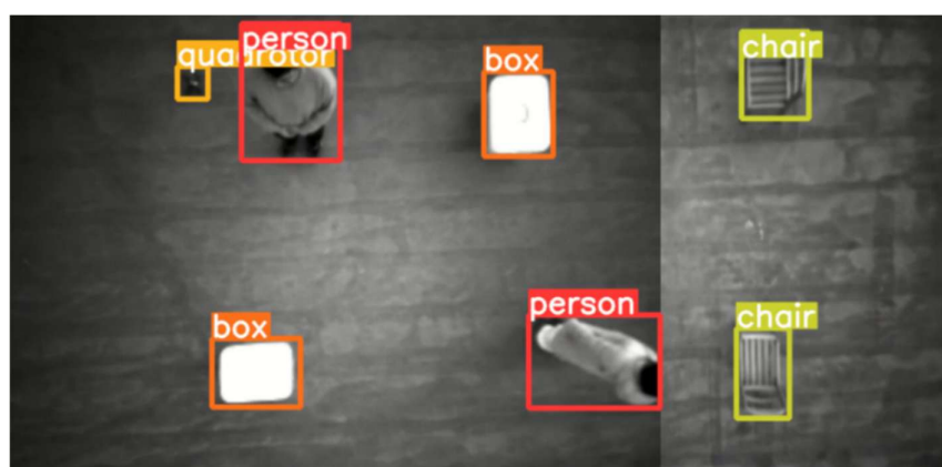
Figure 12. Results of UAV image stitching and object detection.
